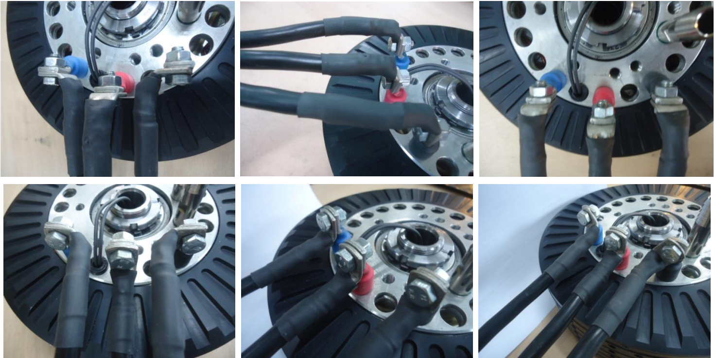
Figure 44: Angular connection of motor connectors to controller cables. It must be isolated with shrink hose!
