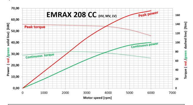
Note 1: for determening peak or continuous power (kW) you should choose motor speed and than read power from chosen power curve (in the left graph side)
